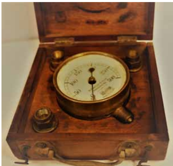
Boiler pressure gauge
